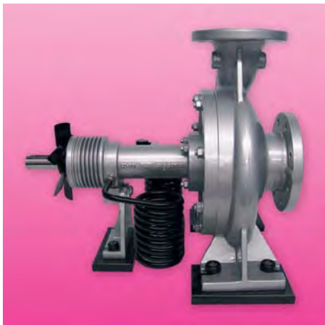
Volute casing pump – Hot oil design type NKX with single mechanical seal for heat transfer oil up to 350°C (662°F).
